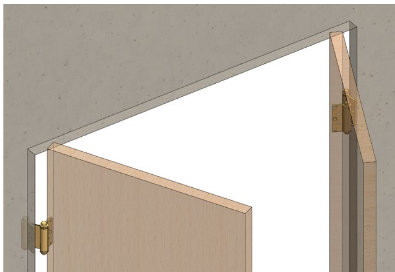
Two hinges per door panel
